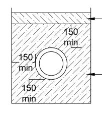
Trench fill under roads to conform with Highways requirements.
