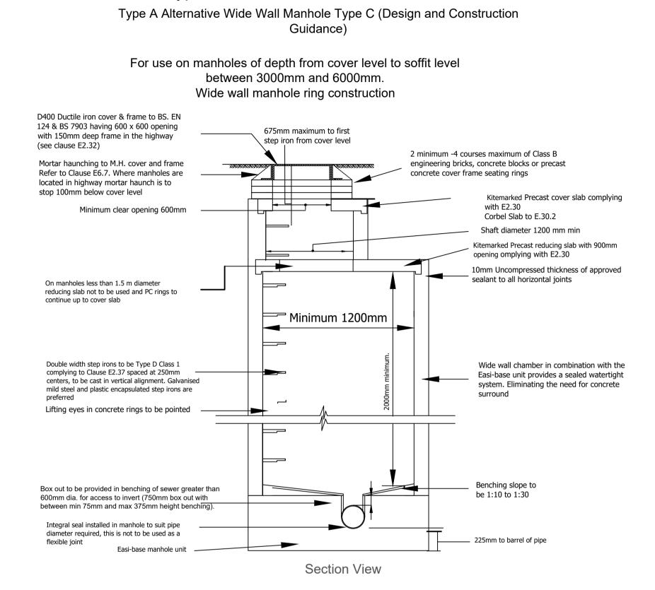
Typical Widewall Manhole Construction
