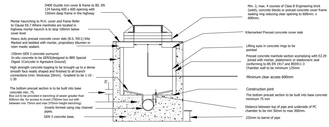
Where Type C manholes are 1500mm or greater in diameter a 1220mm x 675mm clear opening is required with a double twin 600mm x 600mm covers is required.
